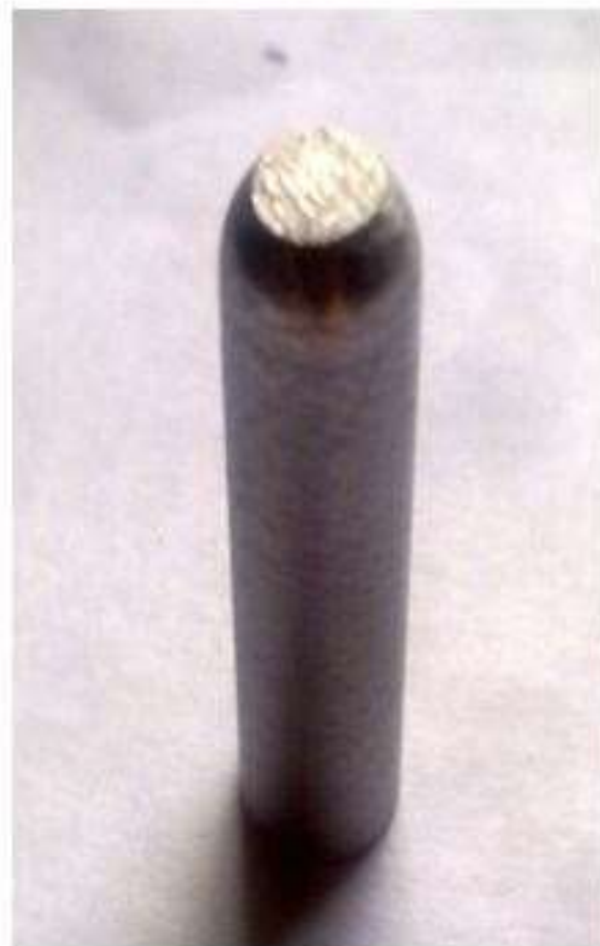
Fig 3 Pin specimen made of D2 steel (after wear)
