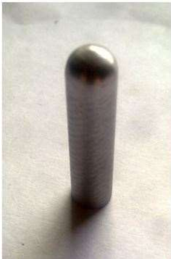
Fig. 2 Pin specimen made of D2 steel (before wear)
