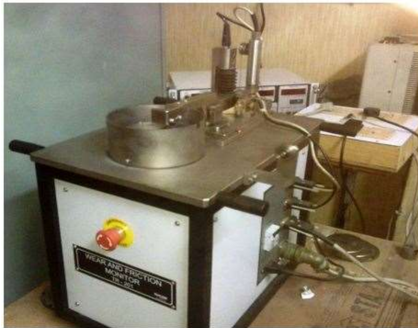
Fig. 1 Wear and Friction monitor TR-201 (Courtesy: Metallurgy Lab, SLIET, Longowal)
